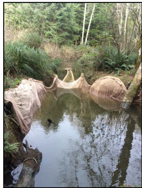
FIGURE 1. Trapnet and livebox set up at confluence of Elk Flats channel and Ecola Creek mainstem.
